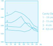
Vari panel can be tuned between 50Hz and 100Hz by simply rotating its wooden top. Recomended for rooms smaller than 10m<sup>2</sup>
