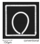
SCANahead control ensures precise traversal of the defined set circle even at high circle speeds. This substantially simplifies correct processing of circles and boosts productivity thanks to increased trajectory velocities.
