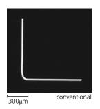
SCANahead control fully exploits the galvos' dynamic performance potential. Hence traversal of 90° corners at a wide range of speeds produces far less corner-rounding. Additionally, SCANahead allows faster traversal of corners having identical radii.
