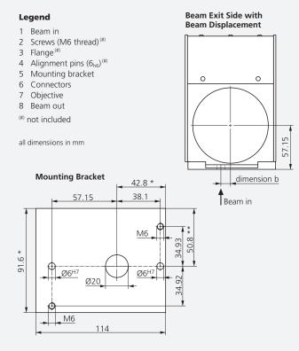
Standard mounting bracket (10 mm aperture): rectangular, without cut-out
