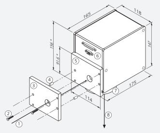
Denoted dimensions refer to the **standard housing** type with 10 mm aperture. Variations in height and depth of the housing are possible; also housings with water cooling have other dimensions.
