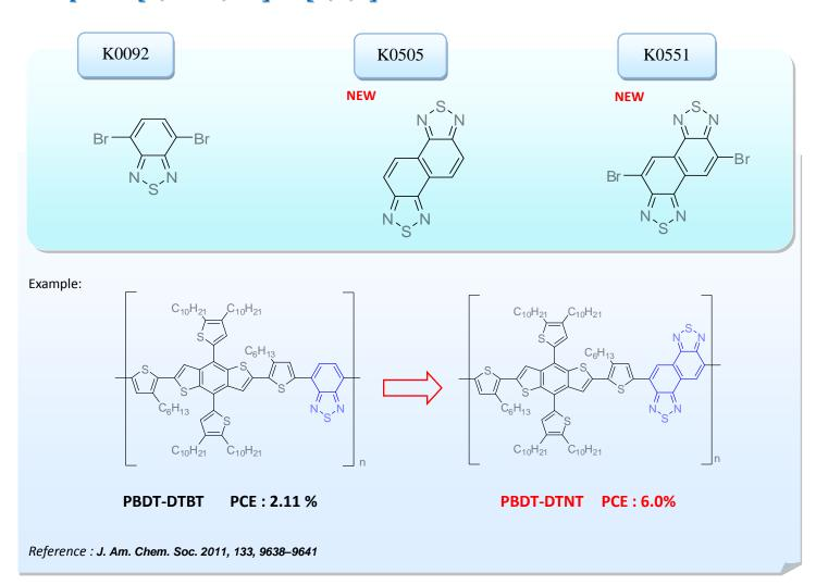
Various donor-acceptor(D-A) conjugated polymers have been developed to achieve high PCEs. 2,1,3-benzothiadiazole(BT) has been proven one of the most promising units for high-performance polymer solar cells(PSCs) materials among the conjugated polymers, and it has used as an electron-deficient receptor widely.
