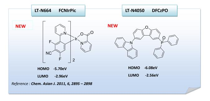
FCNIrPic was designed as a deep blue phosphorescent dopant because a strong electron withdrawing group in phenyl unit of main ligand can induce a blue shift of emission spectrum. The PL emission peak of FCNIrPic was observed at 460 nm with a vibrational peak at 485 nm.
