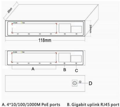
A. 4\*10/100/1000M PoE portsB. Gigabit uplink RJ45 portC. Gigabit uplink SFP portD. DC48-52V
