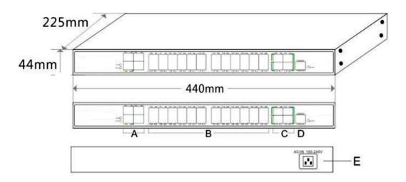
A. 4 \* 10/100/1000M RJ45 Port B. 24\*100/1000M SFP Ports C.4\*1/10G SFP+Ports D. Console port E.Power Input Port AC100-240V,50/60Hz
