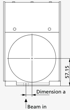
Denoted dimensions refer to the **standard housing type** (with standard mounting bracket).
