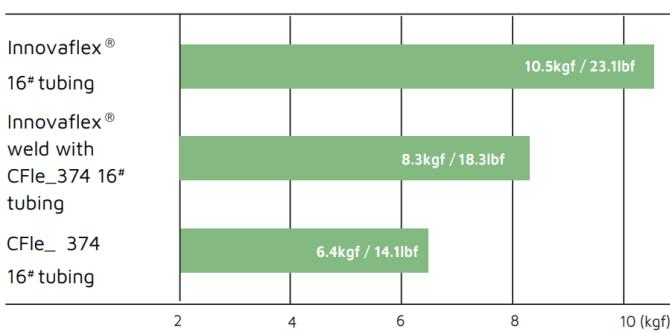
Uses 5 standard 16# size tubings, sterilized under 25kGy Gamma radiation, measure tensile strength after tubing welding by using GE STF-IRc welder.
