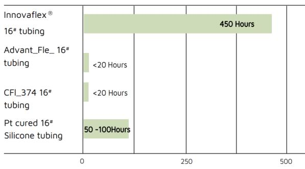
Tests above were conducted by using 16# standard size peristaltic pump tubings, under conditions of 1.5Bar pump head pressure, zero back pressure, water medium and room temperature. A 4 rollers peristaltic pump was used under 600rpm until tube leakage or 30% lower flow rate was observed.
